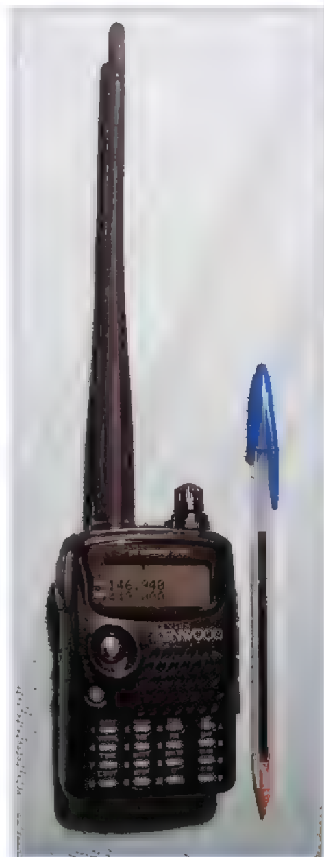
■ FIGURE 1. The Kenwood TH-F6A is a tri-band handheld FM transceiver for the 144, 222, and 440 MHz ham bands. Lots of buttons and menus make it a challenge to use.
